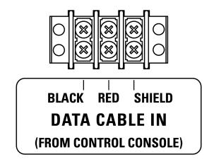
You may purchase data cable from Electro-Mech, or you may source it elsewhere. We recommend (and supply) cable that is rated for direct burial. It includes two insulated 22 AWG stranded conductors (red and black), along with a non-insulated conductor, all wrapped by a braided or foil shield. This document will discuss, in a few pages, what the other end of this cable is connected to.
